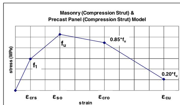
Figure 4. Compression strut model for masonry infill walls strengthened with RC precast panels.
