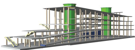
Durrees Parking Lot Reinforced Concrete Frames Total Area: 15.000 sq. meters
