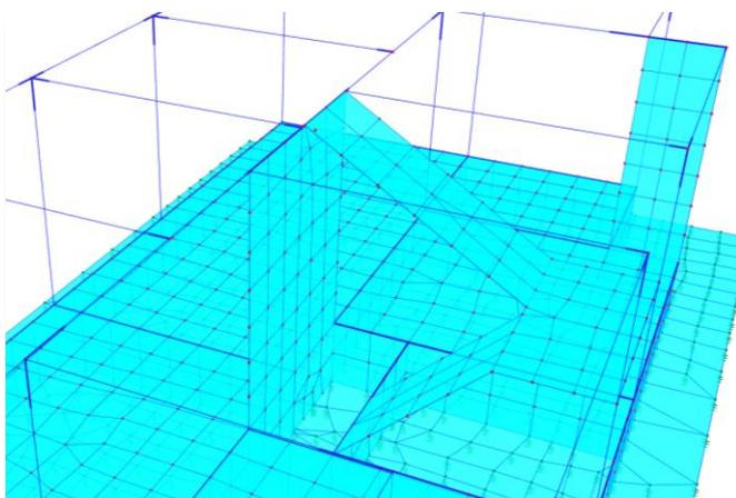
*Analytical model of the building. Slabs are not meshed with the building. Staircase is connected to the shearwall at the top and subbasement wall at the bottom.*
