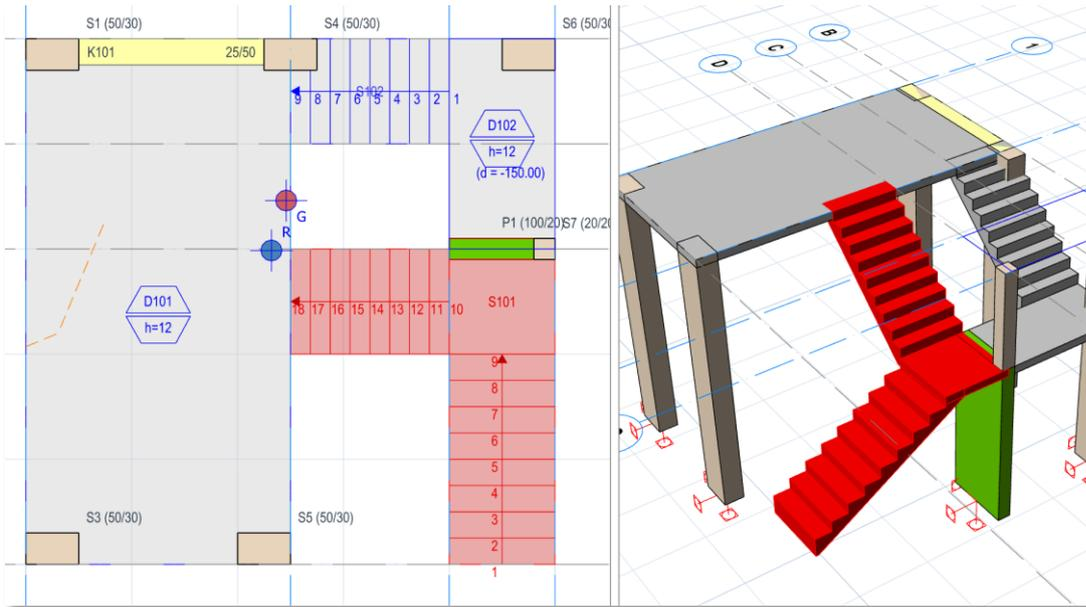
This type is similar to straight staircases with landing. Insertion procedure and the governing parameters are the same with straight staircases with landing.
