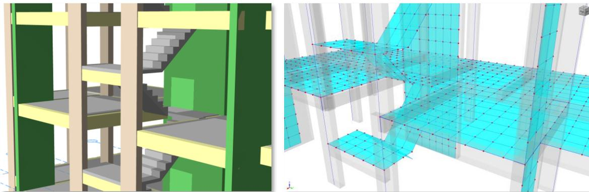
You can see the same staircase automatically connected to the subbasement beam at the foundation level.
