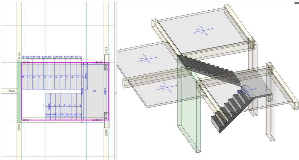
*The view from the staircase editor. See how the staircase has unequal flights*
