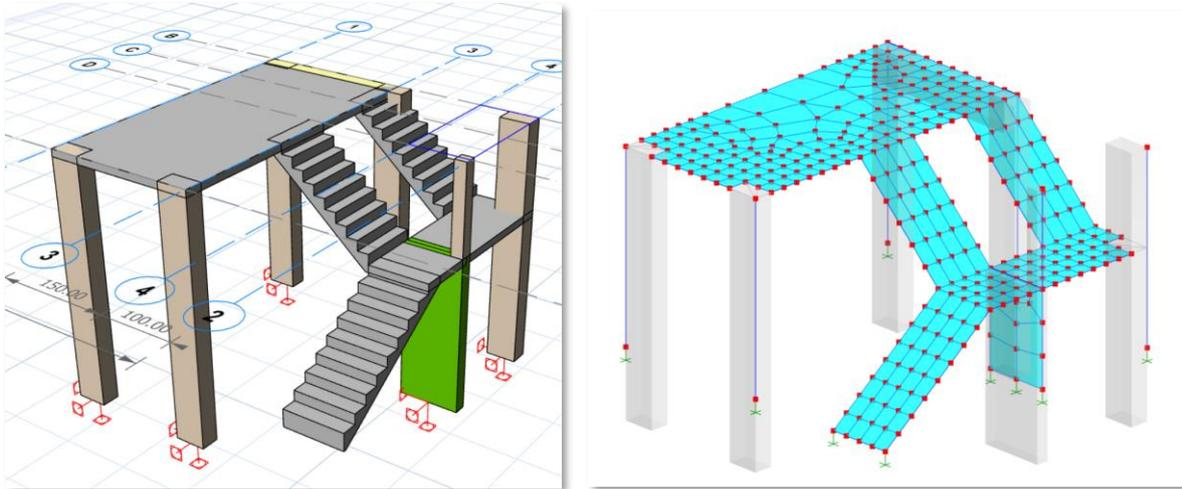
The following images show a U-shaped staircase with two landings placed inside a corewall. ProtaStructure will identify the supports and mesh the staircase compatibly with the shearwalls.
