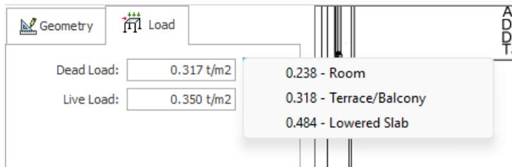
The predefined **Self-Weight** and **Additional Dead Load** is automatically considered in the 'G' or 'D' load case, whereas, the **Live Load** will be automatically assigned to 'Q' or 'L' load case.
