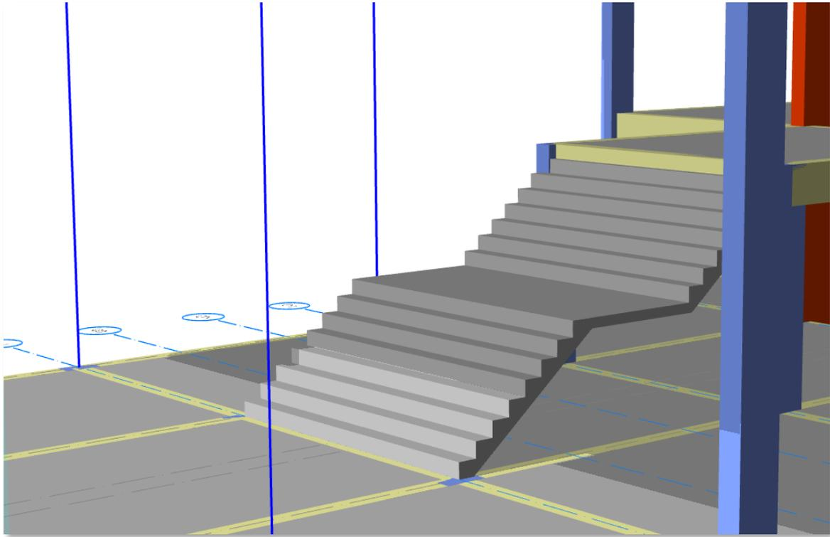
As the name implies, this type is similar to straight staircases, but with an additional landing. The insertion and loading procedure is exactly the same as straight types. There are additional fields that governs the landing and the second flight.
