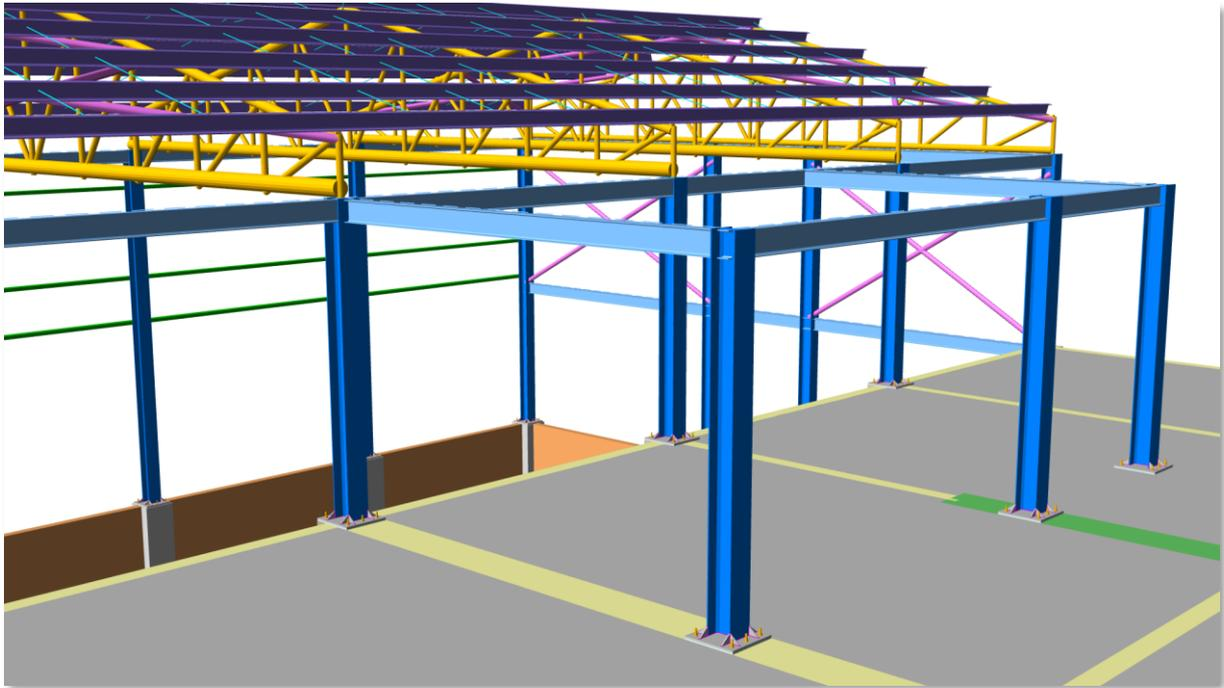
ProtaStructure will automatically recognize the member under the steel column, that will constitute a support for the base plate.
