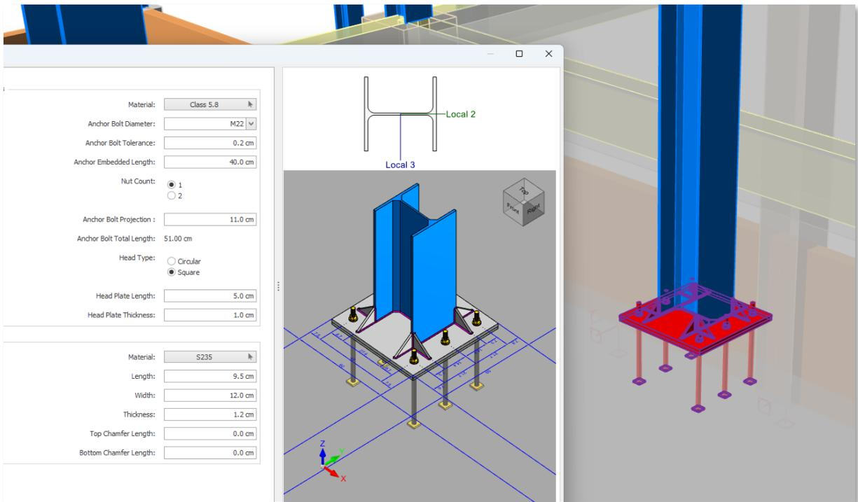
*Base plate sitting on a thick slab at the upper storey*
