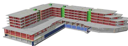
Onyx Ankara Residential Complex Reinforced Concrete Frame Structure Total Area: 20.000 sq. meters
