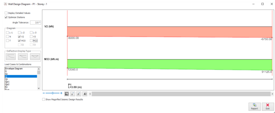
Base shear and moment diagrams of P1 corewall under Q load case in ProtaStructure
