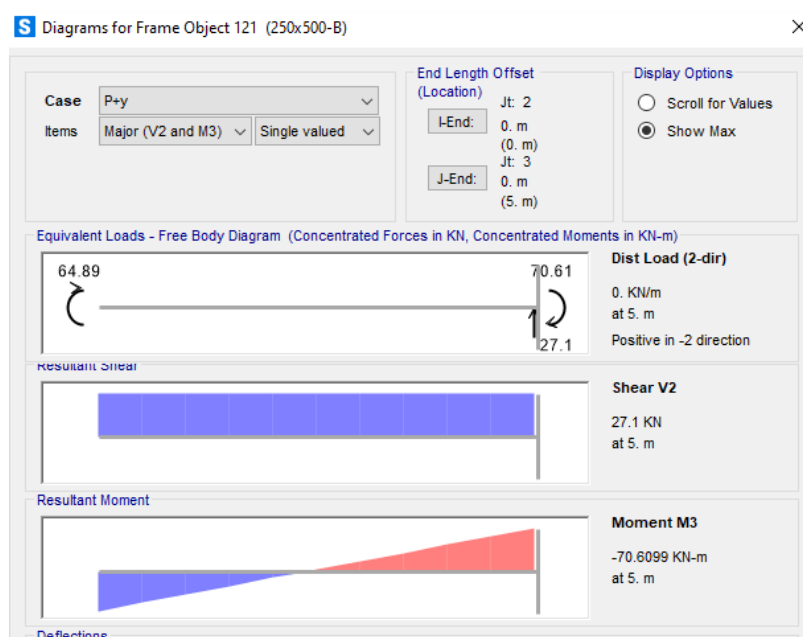
Moment and shear diagrams of the beam K-101 in SAP2000
